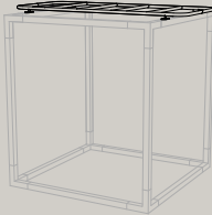
LEV901 1160 × 2640 × 88, Ø40 ladders on the roof
